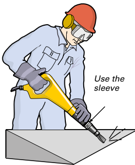
Because the shockwaves in them cause vibration, the chisel or die should never be held.
