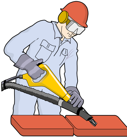
Chipping hammer RRD with dust extraction used in building industry.
