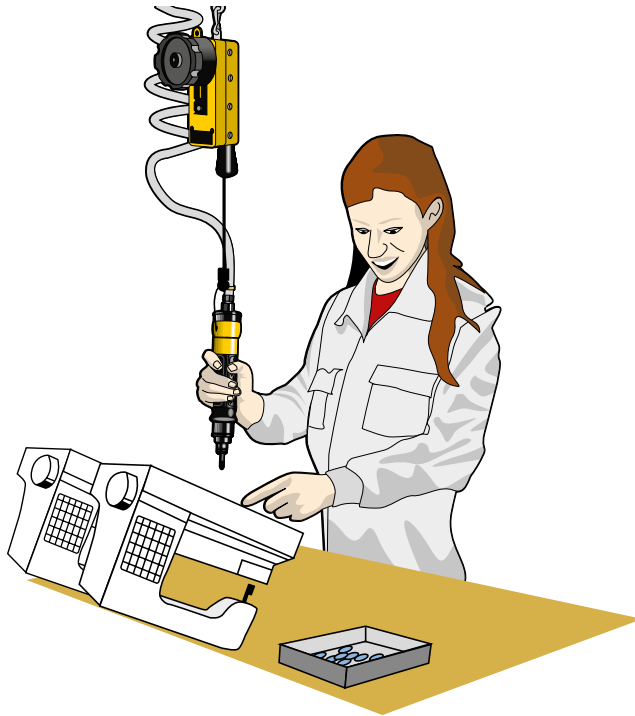
Bench assembly of small electric devices is a typical application for screwdrivers supported in balancers.
