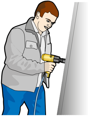
Never hold the socket on impact wrenches or impulse tools.
