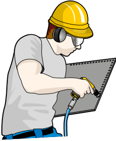
Riveting is typical of an operation that generates a great deal of process noise.
