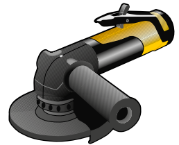
Angle grinder LSV 38 with a support handle with a small extra weight stiffly mounted on the tool to reduce vibrations.
